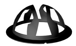
Computer-generated shadow mask within the SPN1 ensures that one of the 7 thermopiles is always exposed to the full solar beam and one is in full shade regardless of the sun's position.
