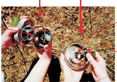
SKPM 1445 Specimen holding adapter. Choice of 3 sizes. Change using the 4 screws
