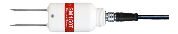
The SM150T's accurate and stable measurement (± 3% for 0-70% VWC range), simple 0-1 V output (moisture), and low power (18 mA for 1 second) makes it an ideal sensor for system integrators.
