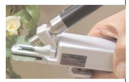
The Standard PAR Clip is designed for one hand operation. The underside opening mechanism prevents the weight of the fibre optic cable opening the PAR clip unexpectedly.
