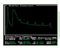
**Kinetic test:** Advanced quenching analysis using Puddle and Lake measuring parameters. Ultra stable light source ensures accurate measurements. NPQ, qP, qN and Y(II). Kramer lake model Y(II), Y(NPQ), Y (NO), and qL Hendrickson lake model Y(II), Y(NPQ) Y(NO) and NPQ.
