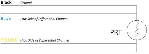
**Note**: as shown in the schematic, the 4-wire PRT can be directly measured. The black and blue wires are electrically connected to one side of the PRT while the yellow and white wires are electrically connected to the other side of the PRT.
