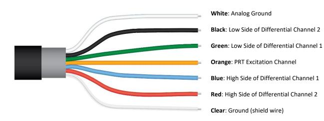
Measurement of PRT resistance is very similar to measurement of thermistor resistance, where a half-bridge measurement is used. An excitation voltage is input across the bridge resistor and an output voltage is measured across the PRT.
