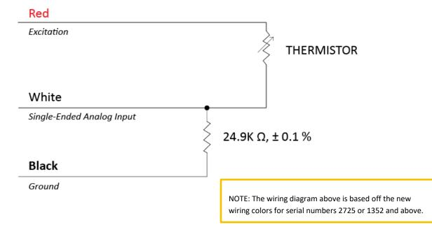
Measurement devices (e.g., datalogger, controller) do not measure resistance directly, but determine resistance from a half-bridge measurement, where an excitation voltage is input across the thermistor and an output voltage is measured across the bridge resistor.
