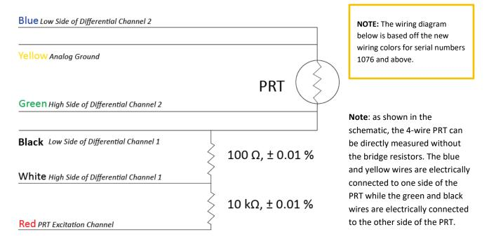
An excitation voltage of 2.1 V DC is recommended to minimize current drain, while still maintaining an adequate voltage signal. However, other excitation voltages can be used. Decreasing the excitation voltage will decrease current drain but will also decrease output voltage. Increasing the excitation voltage will increase output voltage but will also increase current drain.
