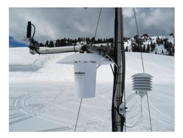
Top left: SP-230 Heated Pyranometer Center: TS-100 Fan Aspirated Radiation Shield Right: RM Young 41303 Static Solar Radiation Shield.
