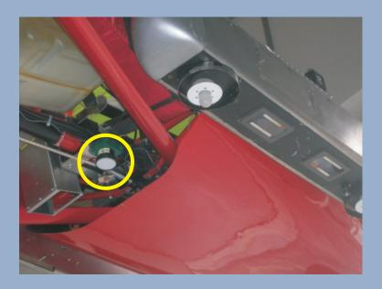
Circled above is the Skye sensor fitted to the small aircraft, while below is a photo taken from the aircraft in flight, showing its surroundings.
