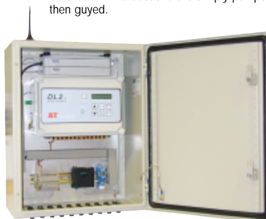
DL2e Logger, GSM modem and antenna, 12V wiring kit and relay, solar power regulator and LBK1 rechargeable battery pack, installed in Weatherproof Enclosure type M2-ENCL.
