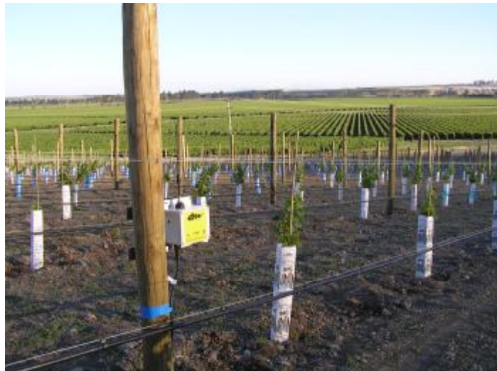
The latest generation SI.95 Logging Sensor with radio telemetry fitted at Redwood Pass Vineyard, Marlborough, NZ.
