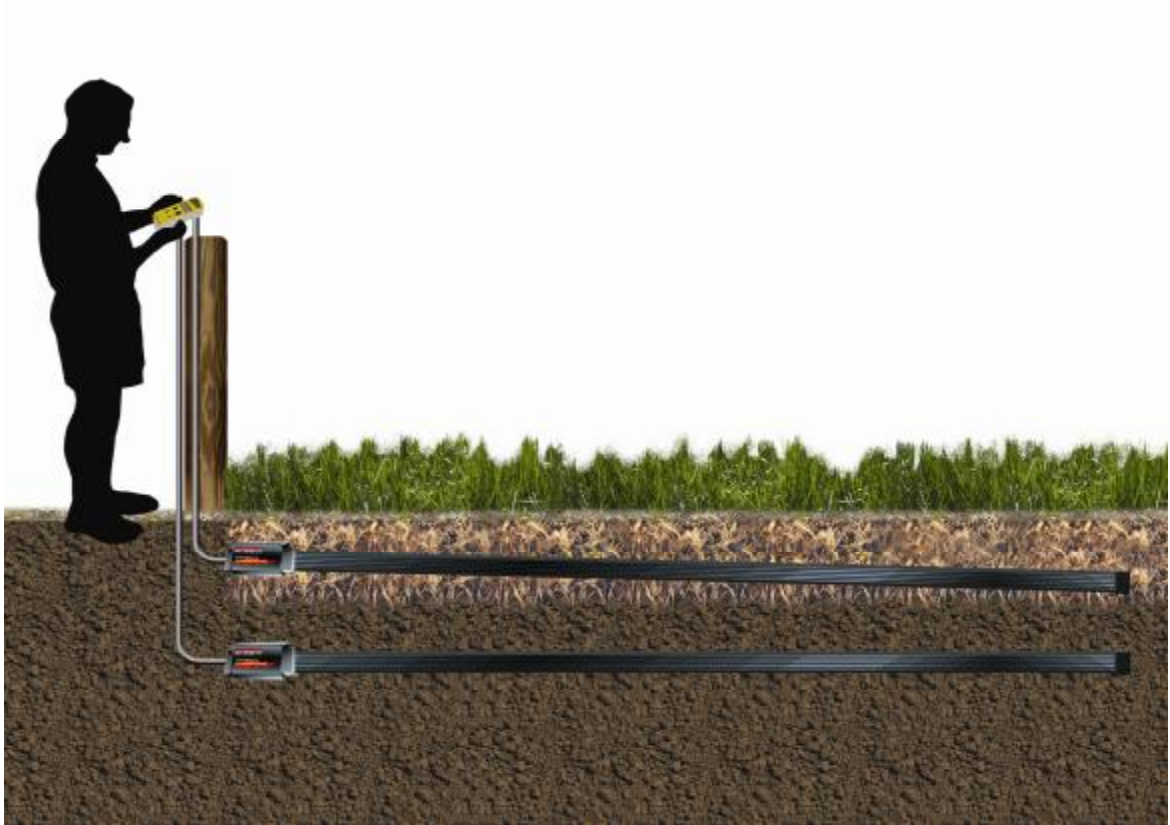
Figure 1: Example of 2 sensor installation in pasture with bottom sensor used to assess over and under-watering
