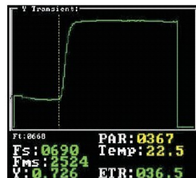
Yield and ETR measuring screen Y is Yield \Delta F/F_m' and Fms is F_m'
