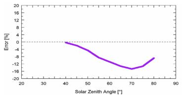
Mean cosine response of four Apogee UV-A sensors. Cosine response was calculated as the relative difference of UV-A sensors from the mean of replicate reference UV-A sensors deployed outdoors. These data are the average of the AM and PM response.
