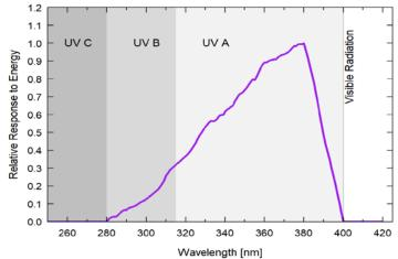
Spectral response estimate of Apogee SU-200 UV-A sensors. Spectral response was modeled from sensitivity of the photodetector and transmittance of the diffuser.
