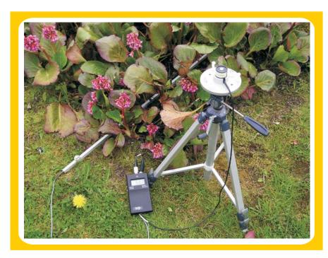
in growth rooms can introduce errors, as the light is usually not constant or not uniform over the whole area. The PAR line quantum sensor instantaneously measures an average of the light falling on its 1m length, hence minimising these errors.
