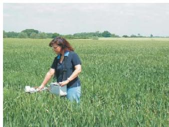
Both the SRS1000 and SRS2000 are highly versatile gas exchange systems. A variety of easily interchangeable plant leaf chambers are available which quickly convert the SRS1000 or the SRS2000 into the most portable research photosynthesis systems ever.
