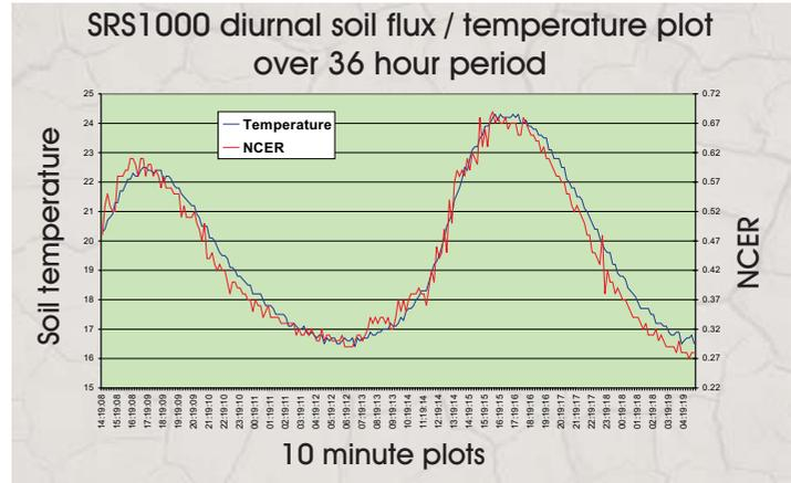
\* The graph shows the stability of CO<sub>2</sub> measurements during a 36 hour diurnal soil flux / temperature plot
