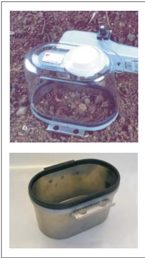
Both the SRS1000 and SRS2000 feature a high quality soil respiration chamber, specifically designed for short-term soil flux measurements. The chamber consists of a lower stainless steel collar and an upper measurement compartment. There are sensors for measuring PAR and soil temperature. Great care has been taken in the design to ensure that no unwanted influences affect the soil flux data:
