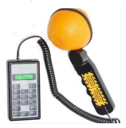
The EFM (Electronic Fruit Size Measure) is a product that makes the measuring of fruit a lot easier. Here's how it works:
