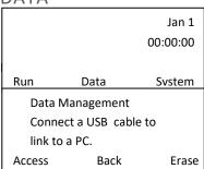
Connect MC-100 to a PC via USB cable or select Access to view data points on screen. Erase to delete data files.
