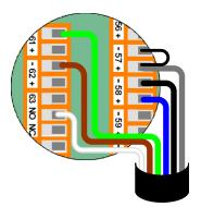
Configure the chosen DL2e logger channels by selecting the appropriate **S3M** and **S3O** sensor types for mineral and organic soils and **S3T** for the temperature sensor type listed in the Ls2Win<sup>5</sup> sensor library.
