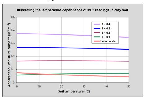
Note: ice has a quite different refractive index from water, so ML3 soil moisture readings cannot be interpreted reliably when inserted into soil below 0°C.
