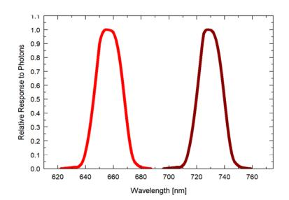
Above: Spectral response of **Red detector (red)** and **Far Red detector (maroon)**.
