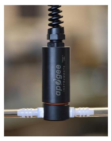
Note: To facilitate the most stable readings, sensors should be mounted vertically, with the opening pointed down and the cable pointed up. This orientation allows better contact between the electrolyte and signal processing circuitry.
