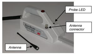
The radio link receiver circuit is built into the probe handle. When the radio system is in use, the probe LED indicates whether or not signals from the BF-RL4 radio transmitter are being picked up.
