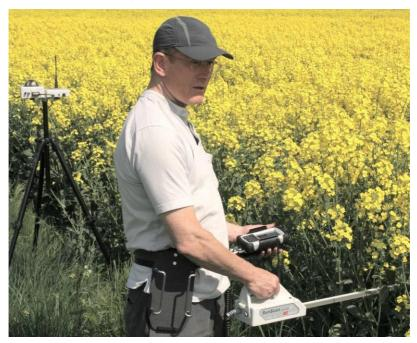
The SunScan radio link is designed to give cable-free operation of the SunScan system in field use. It is no longer necessary to connect the SunScan probe to the reference Sunshine Sensor BF5 by what is sometimes a substantial length of cable (i.e. EXT/8w-xx cables).
