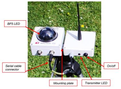
• Connect the transmitter cable to the BF5 serial connector. If you were using the system without radio, disconnect the BF5 to SunScan cable from both the BF5 and the SunScan probe.
